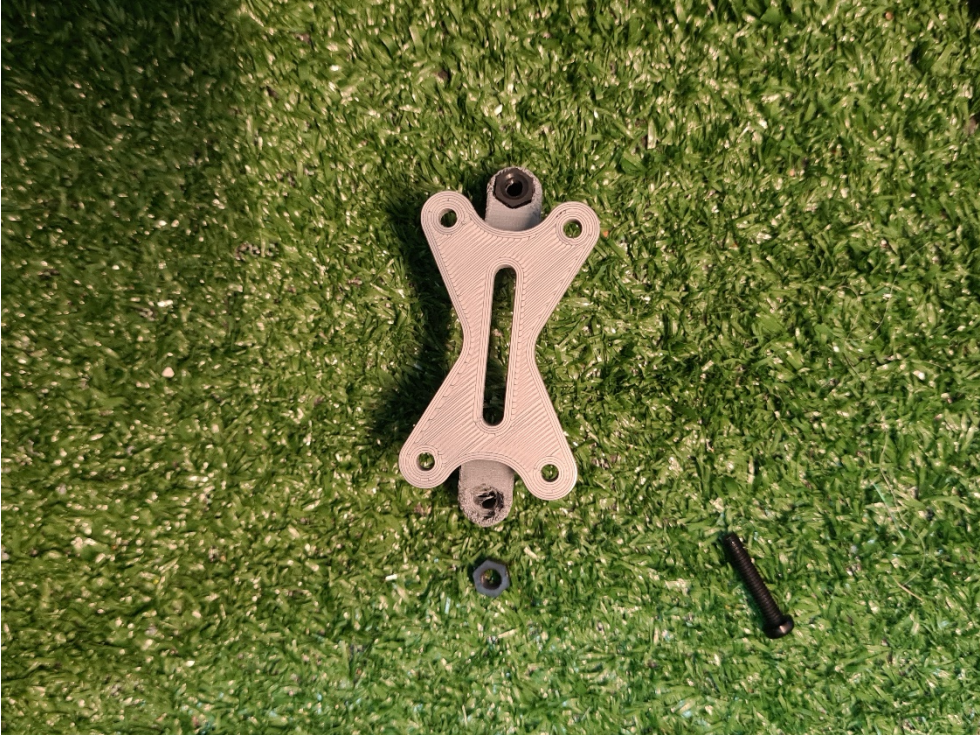
Figure 10. Smart DPV ESC mount, viewed from bottom. Note that the top mounting hole already has black plastic nut installed, while bottom hole has printing artifacts that need to be removed before the nut can be pressed in.
