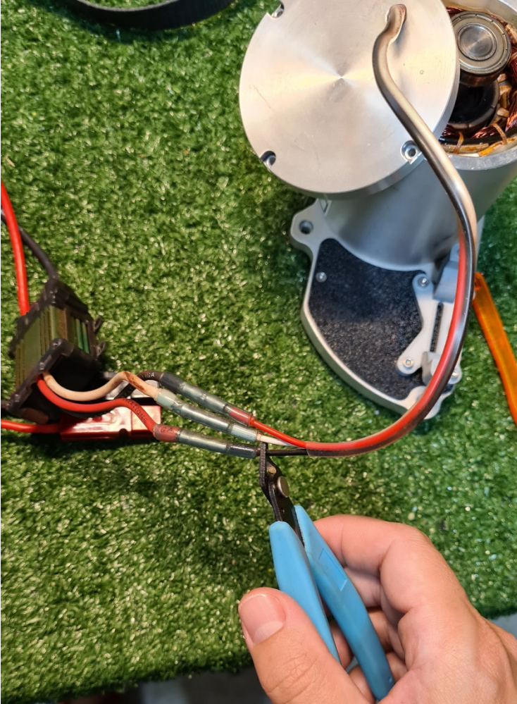
Figure 4. Cut motor wires near solder or butt joints to old ESC.
