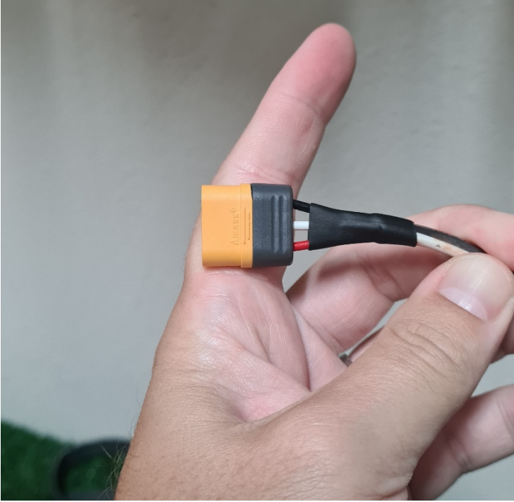
Figure 9. Completed motor plug assembly.
